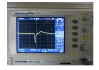
Speaker generates <u>back electromotive force(EFM)</u>, disturbing accurate drive.
