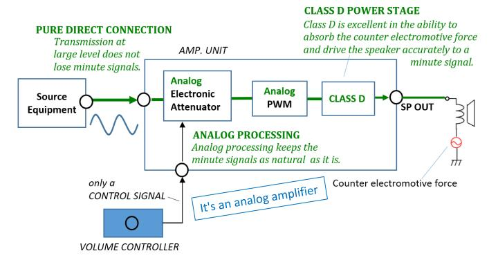
Transmission at large level does not lose minute signals.
