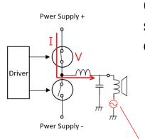
Class D has a very high ability to drive the speakers since the impedance of the final device is very low in principle.
