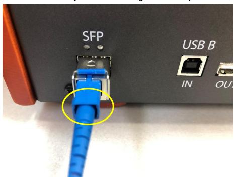
After disconnecting the fiber cable, lower the lever of SFP module as shown below and pull it out.
