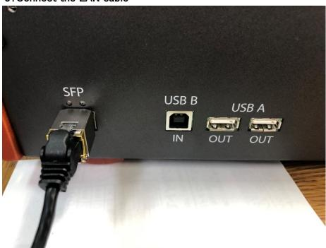
4: Remove the SFP Copper module
