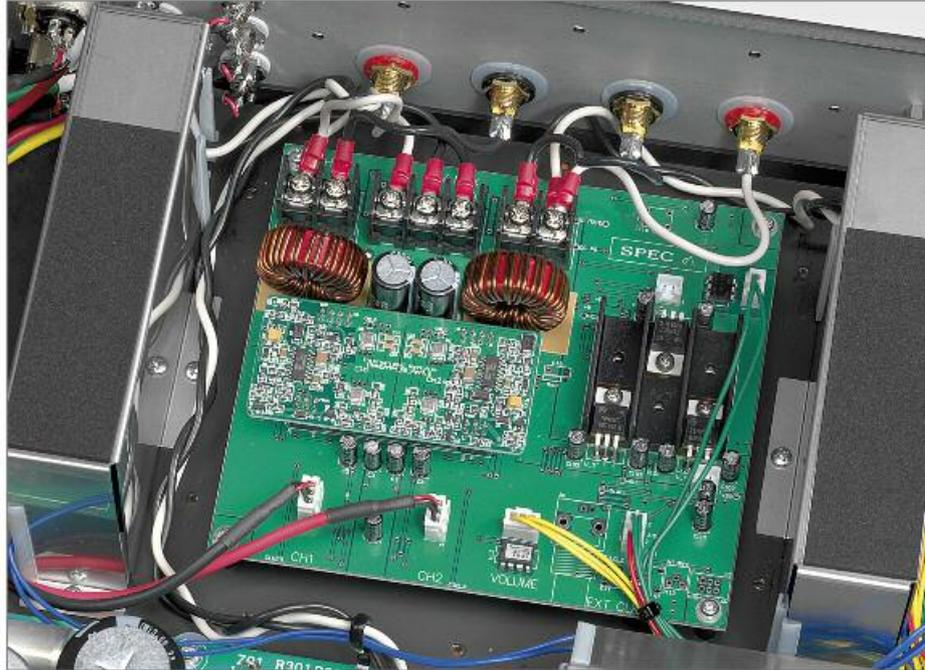
Centre right: The low-pass filter coils were custom developed in house and contain a core of carbonyl iron powder. Since Class-D develops practically no heat, no heat sinks are required, which results in less intensive circuit complexity and shorter signal paths. For this reason, the printed amplifier board which includes power MOSFETs by Infineon Technologies was mounted 'board to board'
