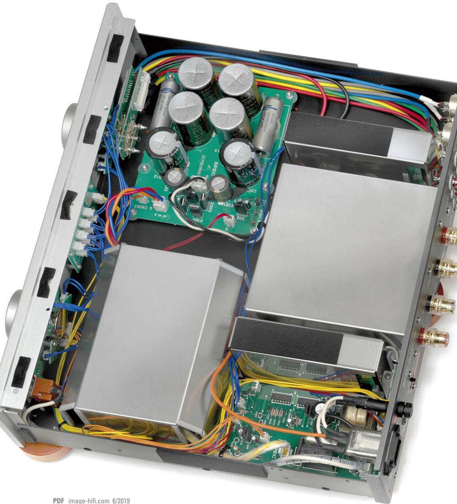
Left: Prevents electromagnetic interference: transformer section, circuit board with low-pass filter and choke circuit as well as the printed circuit boards featuring the pre and power amplifier sections are all shielded individually
